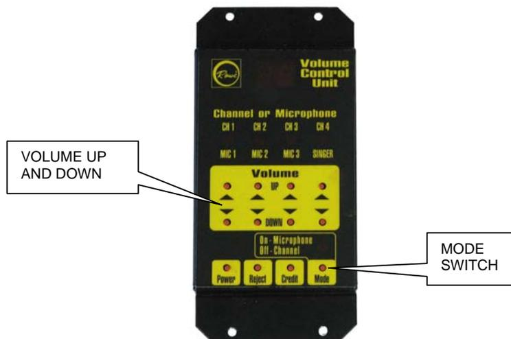
Figure 4 – Presetting the Microphone Volume
